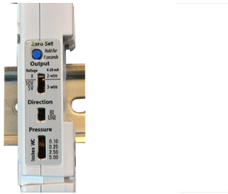
Manual/remote zero. Selectable outputs. Uni/bi directional. Four sub-ranges.
